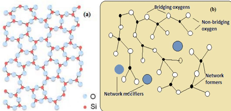
Figure 3 : (a) Silicate network structure, (b) Glass network with modifier
