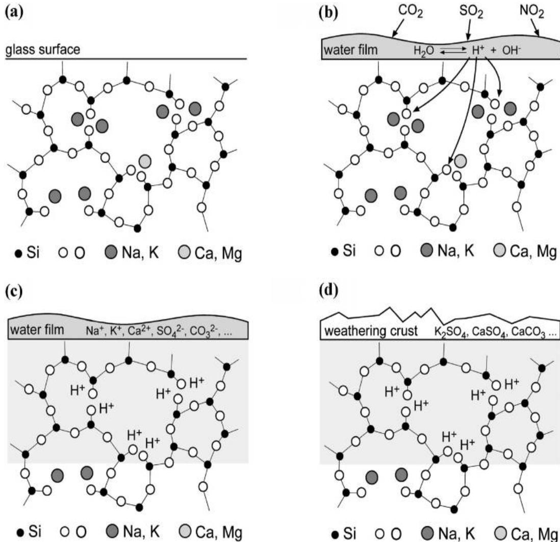
Figure 10 : (a) Glass weathering process starting from a clean surface, (b) a formation of a water film, (c) a leached layer containing Hydrogen, (d) crystalline weathering products on the glass surface.
